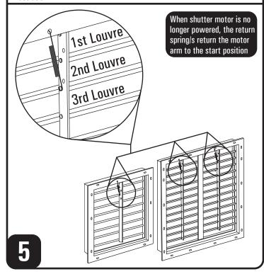
Insert an S-hook into the first available hole below the return spring in each tie bar so as not to interfere with the movement of the return spring. Attach the end of the chain to the S-hook in the tie bar.
