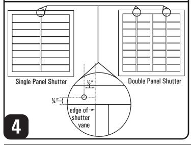
Hook one end of return spring into hole drilled in <u>Step 4</u>. Hook the other end of the return spring around the rivet and spacer for the 3rd louvre from the top. For double panel shutter you will have to do this for each panel. See illustration.
